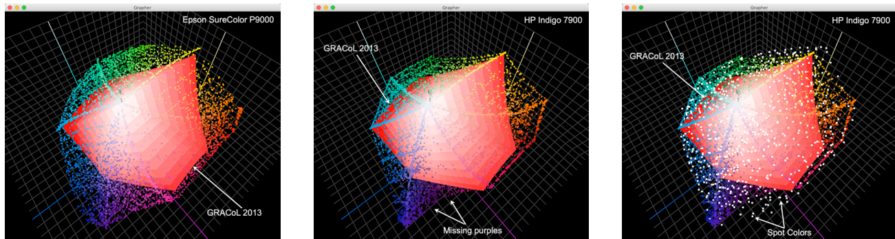
Figure 9: The L^*a^*b^* measurements from all the vendor's characterization data sets, were combined to provide a visualization of the device gamut. Measurements are compared to the GRACoL 2013 gamut, clearly illustrating the gamut expansion due to the added OGV colorants. The Epson P9000 gamut has a gamut that is larger than the Indigo 7900. The Indigo 7900 exhibits “concave” behaviour between colorants and cannot create some purple spot colors. All plots are at the same scale and perspective.
